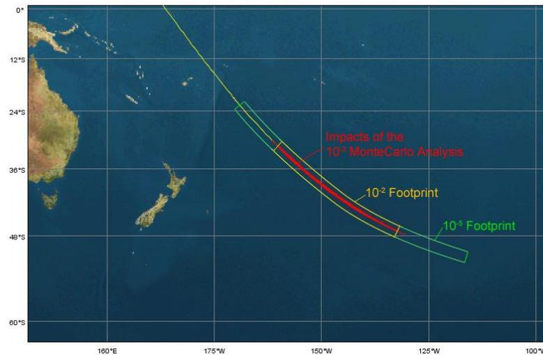
**Fig. 6 Impact points (red dots) of ATV-1 with safety footprints.**
