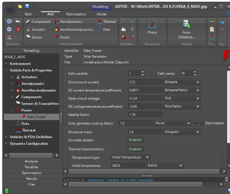
Fig. 3 Solar generator input panel.
