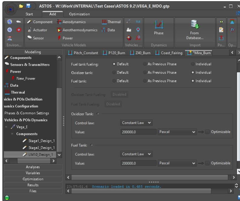
**Fig. 4 Phase-specific definition of tank pressure.**
