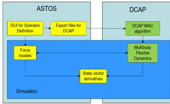
Fig. 14: DCAP and ASTOS interaction framework
