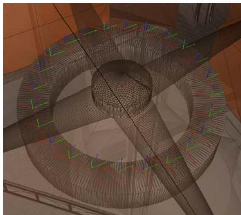
Fig. 4: The stiffness value of each clamp band spring element can be linked to a single static variable
