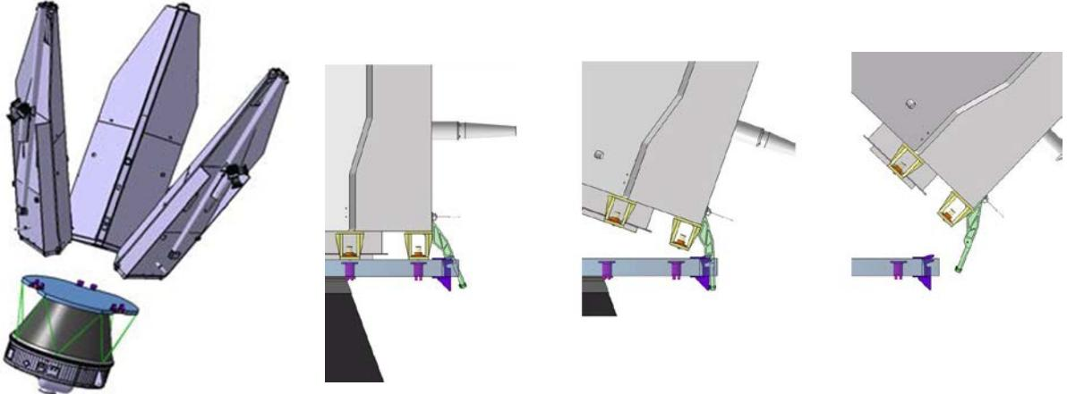
Fig. 6: SWARM satellites separation system
