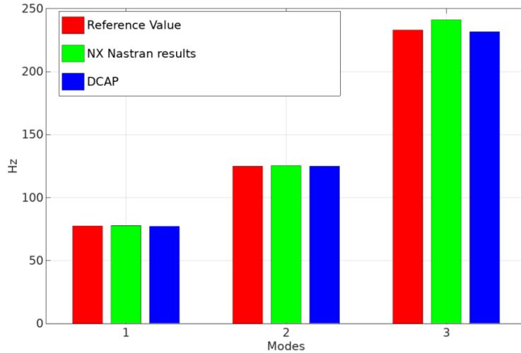
Fig. 13: Comparison of torsional and axial modes with benchmark analytical reference and NASTRAN NX v10
