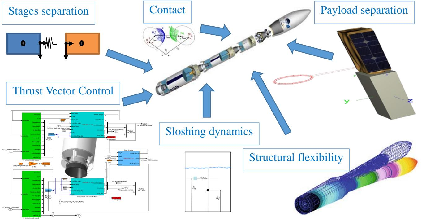
Fig. 2: DCAP launcher simulator features
