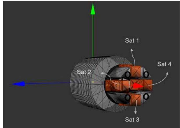
Figure 7. Four satellites mounted on the SSMS structure
