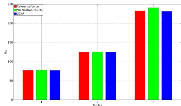
Figure 4. Benchmark of the torsional and axial modes between DCAP, NASTRA NX and reference computations
