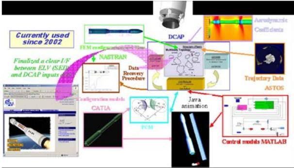
Figure 2. ESA launcher multibody dynamics simulator: general overview
