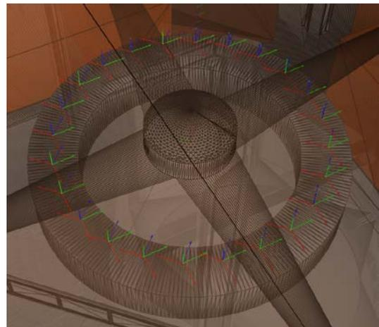
Figure 8. Springs located on the clamp band diameter
