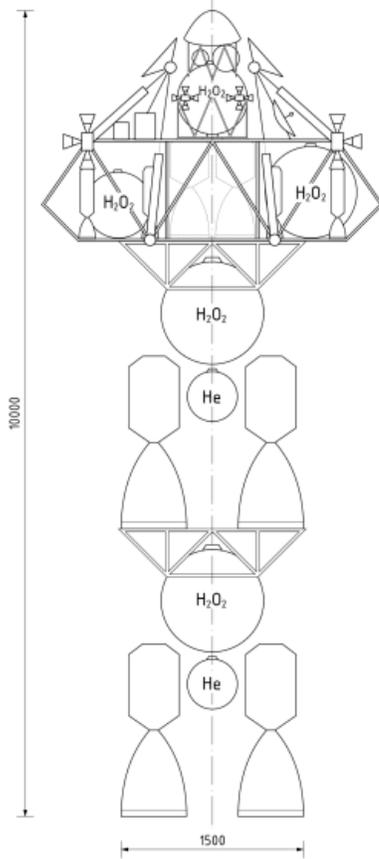
Fig. 7: 3-stage landing vehicle
