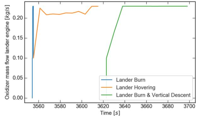
Fig. 8: Oxidizer flowrate during landing phases
