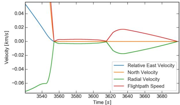
Fig. 9: Velocity during landing phases
