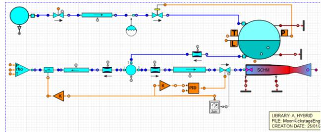
Fig. 5: Example of modelling a pressure-fed hybrid rocket motor with ESPSS
