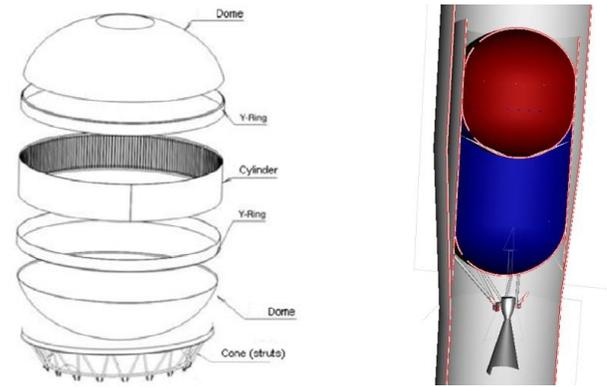
Fig. 4: Substructures (cylinder, dome, cone, struts) (left) and stage under fairing configuration of ASTOS (right)
