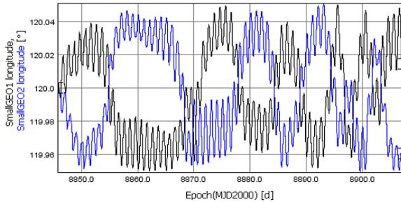
Figure 6. Longitude evolution with a 15 km minimum inter -satellite distance constraint
