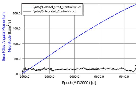
Figure 4. Constraint on S/C angular momentum vector
