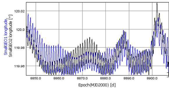
Figure 5. Longitude evolution in absence of inter-satellite distance constraint
