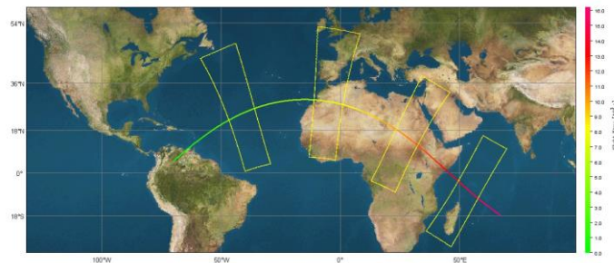
Fig. 4: ASTOS map plot showing snapshots taken at each hour along a MEO.
