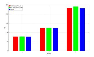
Figure 4. Benchmark of the torsional and axial modes between DCAP, NASTRA NX and reference computations
