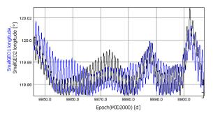
Figure 5. Longitude evolution in absence of intersatellite distance constraint
