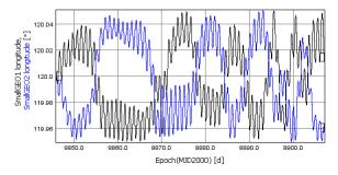
Figure 6. Longitude evolution with a 15 km minimum inter -satellite distance constraint
