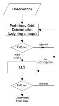
Figure 1. Orbit determination algorithm diagram
